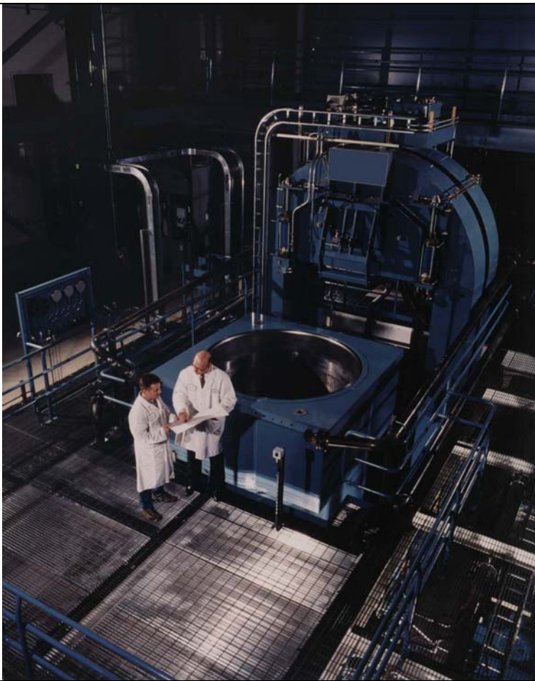
This 1.63 meter diameter HIP unit in Camas (Washington) is an example of the type of large, sophisticated equipment needed to process parts for the ITER project in a cost effective manner.
